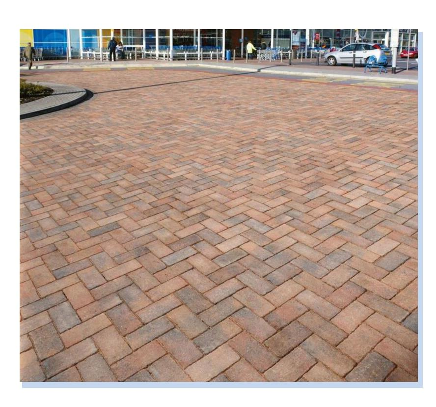
Concrete block paving 'Burnt Ochre' for carriageway crossings
