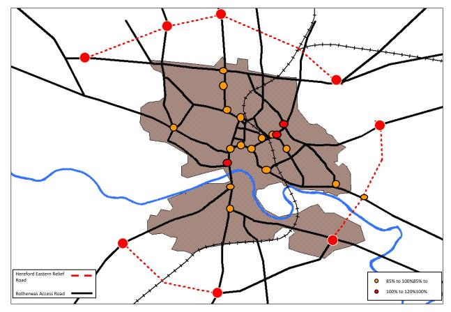
Figure 9.3 Junctions operating at >85% of capacity – AM Peak Scenario 3
