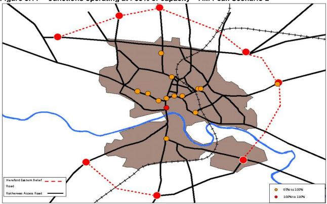
Figure 5.11 Junctions operating at >85% of capacity – AM Peak Scenario 2
