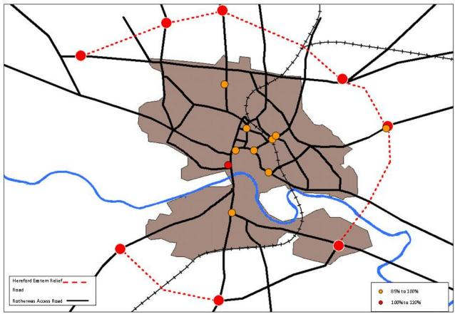
Figure 9.5 Junctions operating at >85% of capacity – AM Peak Scenario 4
