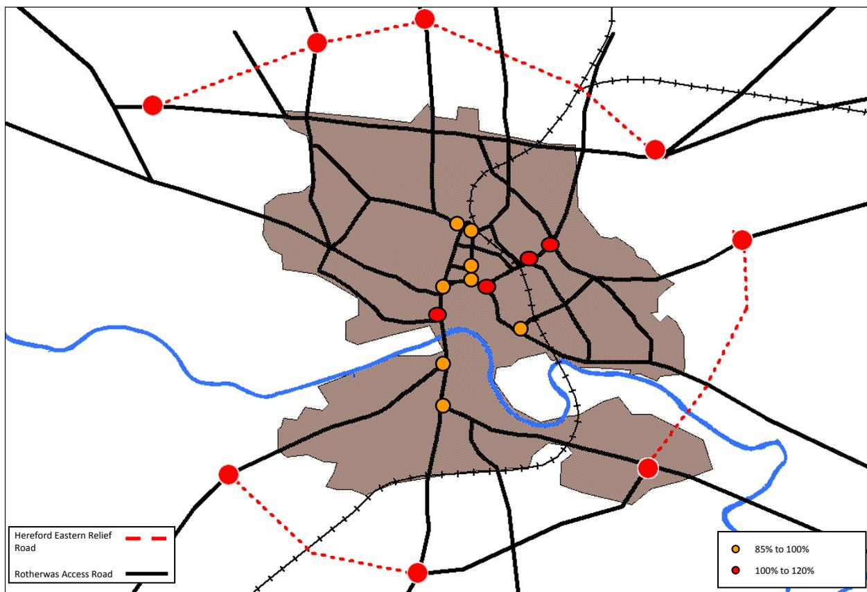
**Figure 9.5** Junctions operating at >85% of capacity – AM Peak Scenario 4
