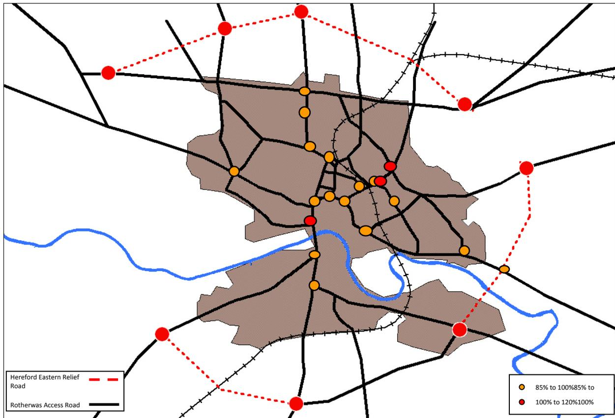
**Figure 9.4 Junctions operating at >85% of capacity – PM Peak Scenario 3**
