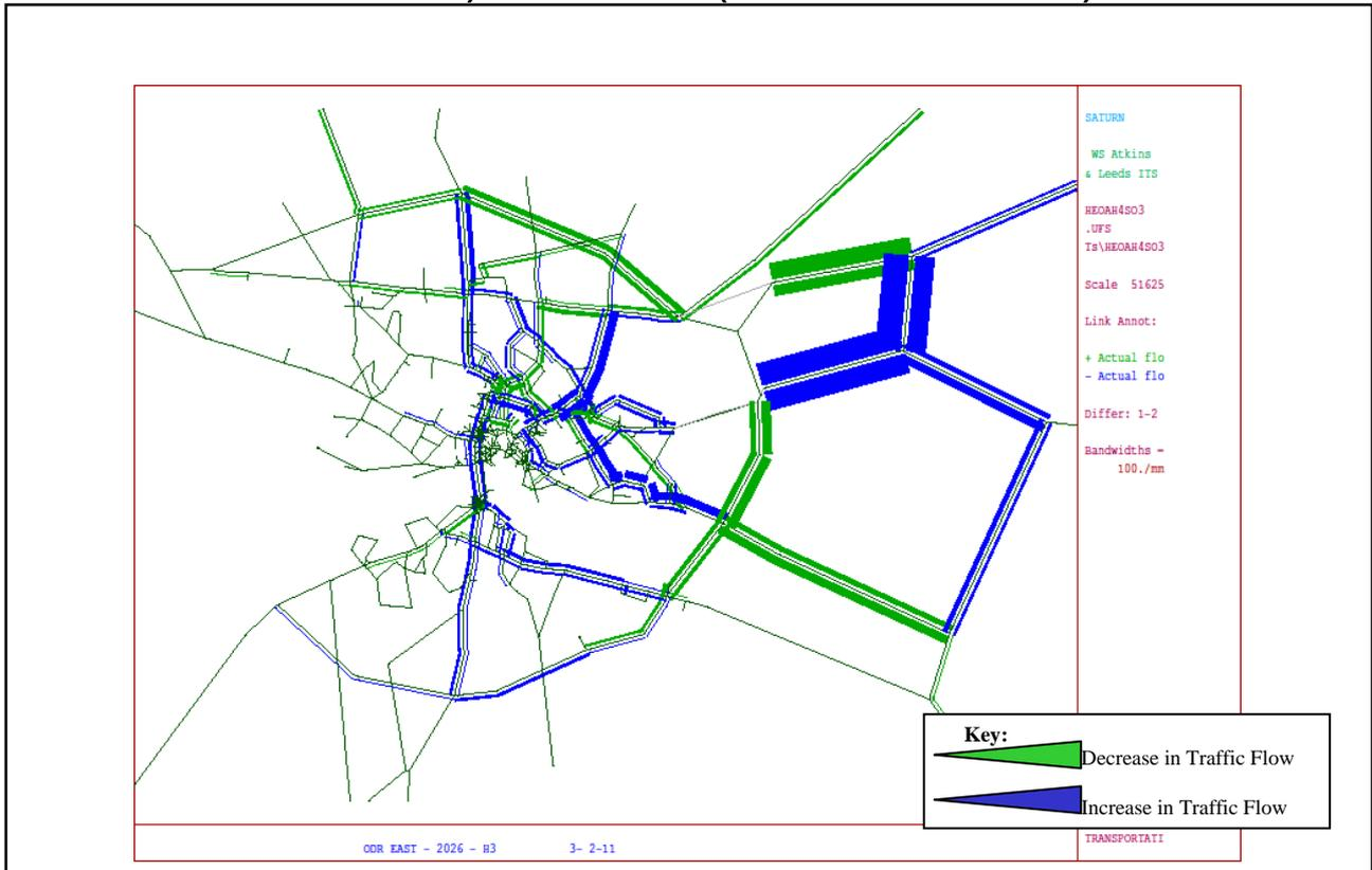
**Figure 5.6** Difference in traffic flows between Scenario 1 (Eastern corridor without a Lumber Lane link) and Scenario 2 (with a Lumber Lane link) – PM Peak
