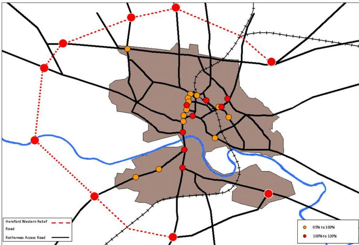
**Figure 5.9 Junctions operating at >85% of capacity – AM Peak Scenario 1**
