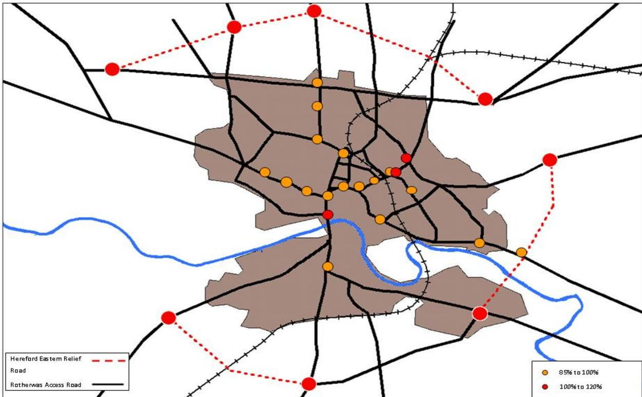
**Figure 5.10 Junctions operating at >85% of capacity – PM Peak Scenario 1**
