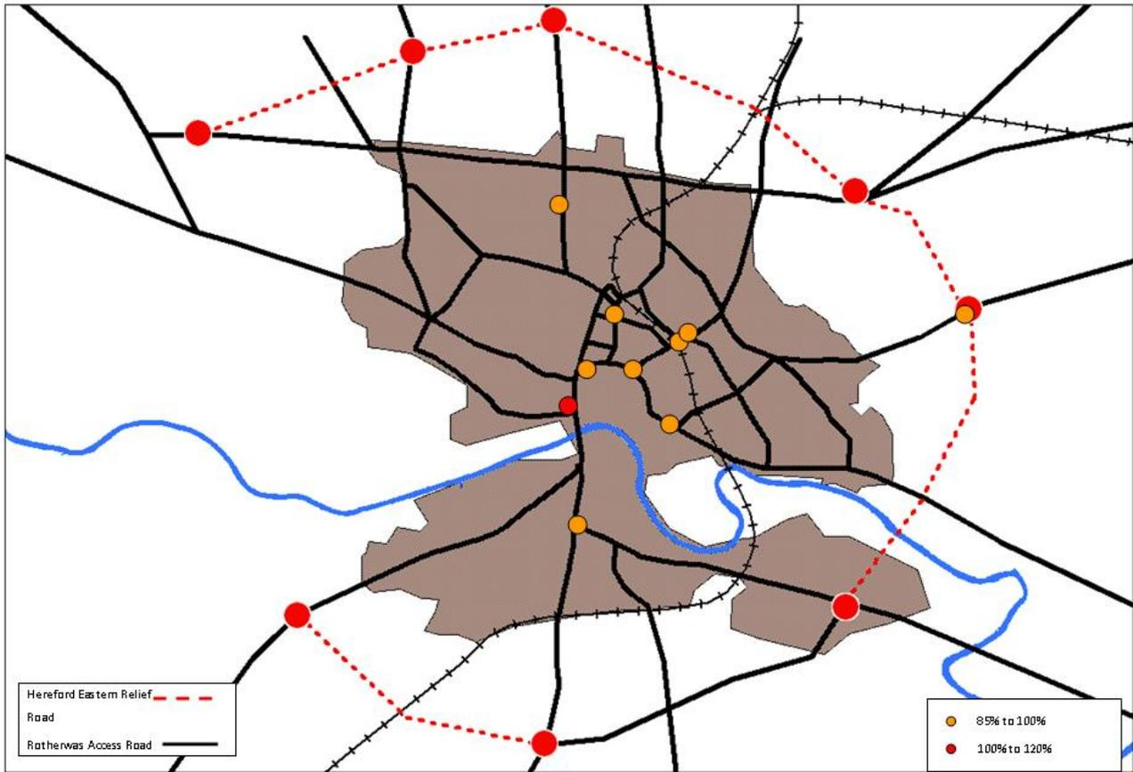
**Figure 9.6** Junctions operating at >85% of capacity – PM Peak Scenario 4
