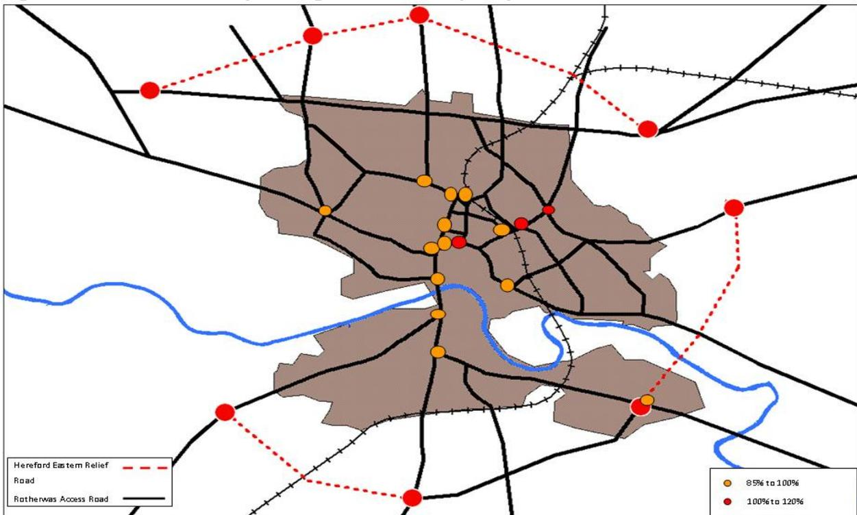
Figure 5.11 Junctions operating at >85% of capacity – AM Peak Scenario 2
