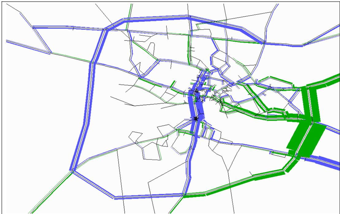
Figure 11: PM 2031 Traffic flow difference plot: Scenario 6 vs Scenario 5
