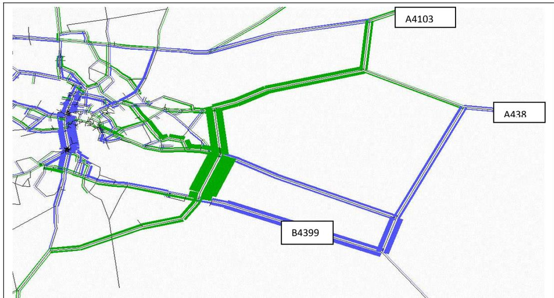
Figure 5: AM 2019 Traffic flow difference plot: Scenario 2 vs Scenario 1
