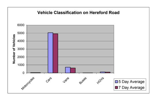
Figure 8 - Classification of vehicles using Hereford Road
