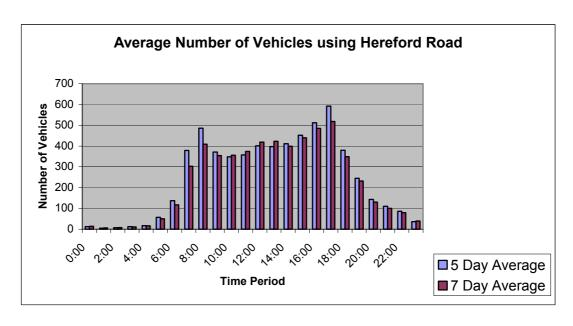
Figure 7 - Hereford Road traffic flow profile.
