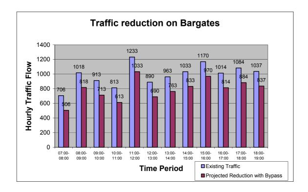
Figure 13 - Impact of Bypass on Bargates
