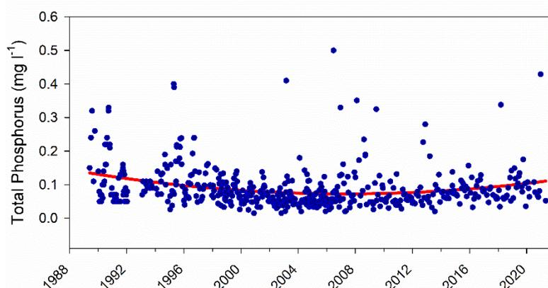
**Figure 10:** The concentration ( $\text{mg L}^{-1}$ ) of total phosphorus (TP) at the outlet of the Wye (Redbrook) from 1989 to 2021 (data provided by Natural Resources Wales). An overall trend line is given. (NB. Data is based on low resolution and inconsistent sampling).
