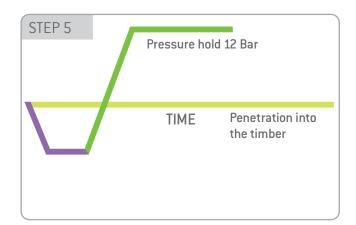
Open Pressure Pump Valve. Start Pressure Pump. Main Flood Valve is closed.
