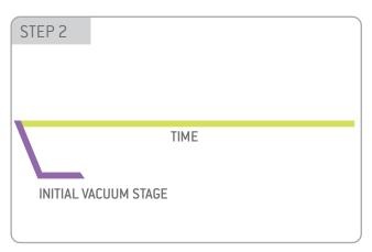
Open Vacuum Valve. Start Vacuum Pump.
