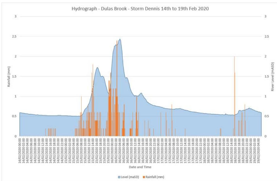
Hydrograph of Dulas brook during Storm Dennis. Data collected using NFM Project river and rainfall monitoring stations
