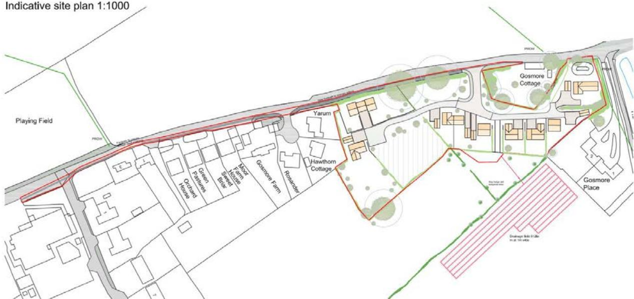
The existing access into the field would be used and upgraded to adoptable standard including and turning head. The road is offset to safeguard the root zone of the large oak trees.
