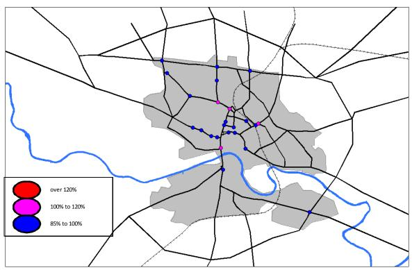
6.171 In the PM Peak model, there are more junctions that are forecast to be operating at greater than 85% capacity than in the AM, again suggesting that some remedial work may be required in order to reduce congestion.
