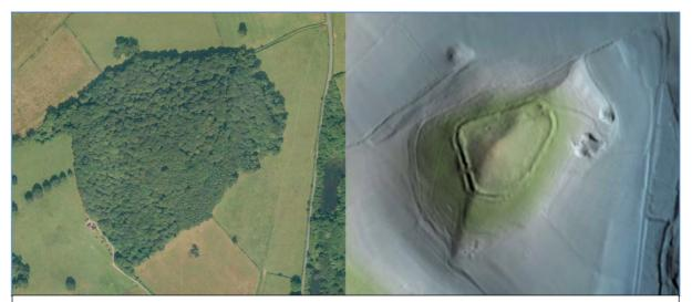
Side by side air photo and LIDAR scan of Pyon Hill penetrating the canopy and showing the ramparts, entrance to the east and later quarrying.
