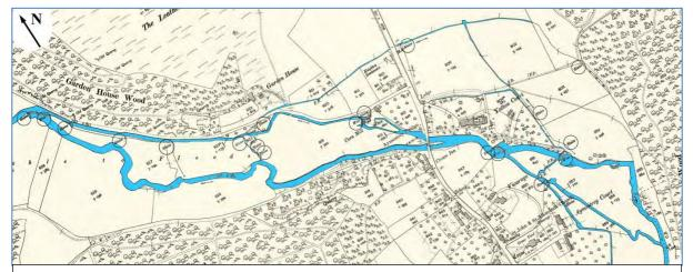
A 1.5 km stretch of the Lugg from Garden House Wood to Aymestrey Court mapped in 1903 showing 19 sluices and weirs along a complex and sophisticated arrangement of leats and channels. The main leat arises from a weir under the wood supplying the Aymestrey corn mill and a channel from its 'tail leat' irrigates the meadows north of Yatton Court. The weir by the Court send water southwards for the meadows either side of the A4110 to Mortimers Cross.
