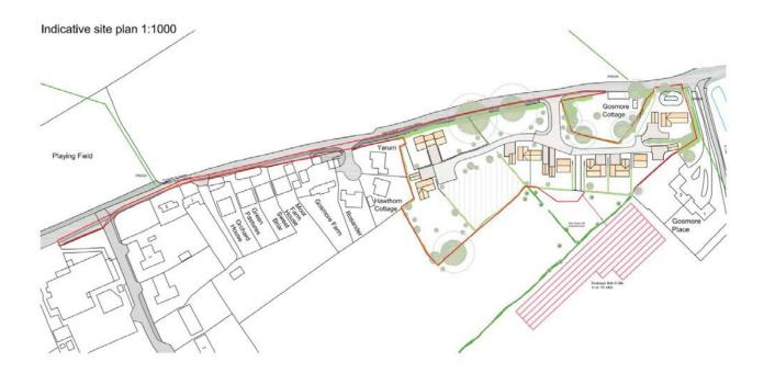
The existing access into the field would be used and upgraded to adoptable standard including and turning head. The road is offset to safeguard the root zone of the large oak trees.
