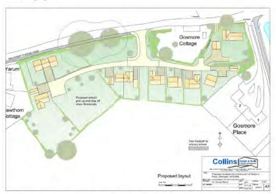
The existing access into the field would be used and upgraded to adoptable standard including and turning head. The road is offset to safeguard the root zone of the large oak trees.
