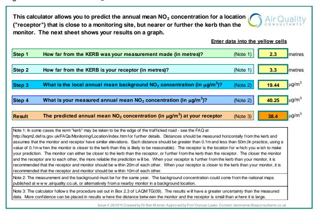
Figure E.2 – Location 10 NO<sub>2</sub> Distance from road calculation
